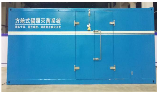
Shelter irradiation system (3MeV/2kW)
