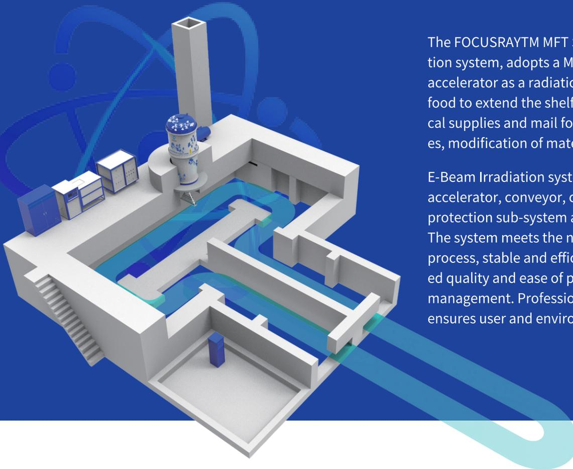
The FOCUSRAY™ MFT Series of E-Beam irradiation system, adopts a Medium -energy electron HV accelerator as a radiation source for process of food to extend the shelf life, sterilization of medical supplies and mail for health and safety purposes, modification of materials for new properties.
